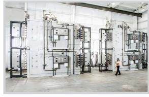
The Microline is the ideal size for research and development and quality control, with continuous processing of up to 8 tows. It is highly customizable and can be configured as a complete system including oxidation ovens, LT, HT, and UHT furnaces up to 2800° C, material handling equipment, and all pre and post treatment process stages found on commercial scale plants.
