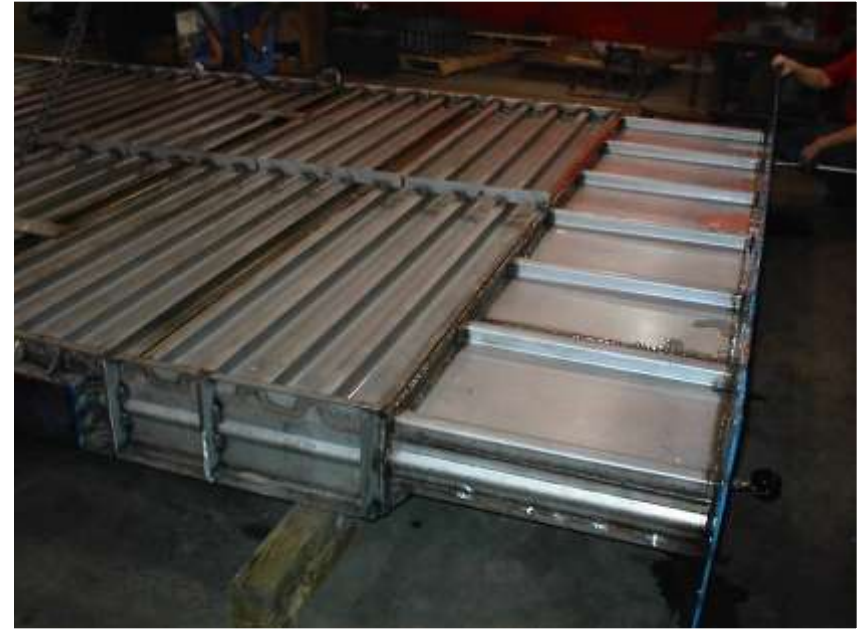
Harper LT Furnace 3 meter wide low-profile muffle
