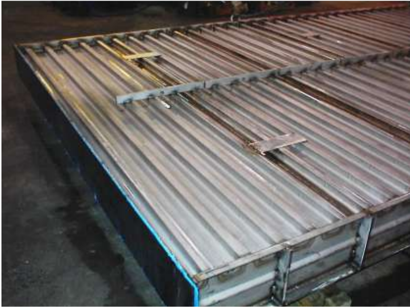
Harper LT Furnace 3 meter wide low-profile muffle
