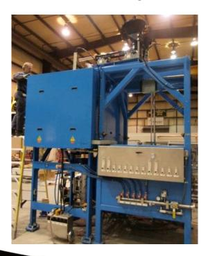
1.25m long, 1 zone 100-150mm ID "tube" 1400°C 2-phase flow Multiple tubes
