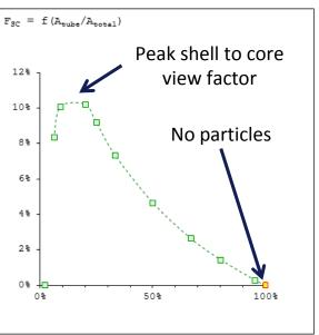
Tube view to core obstructed by dense cloud of particles in shell
