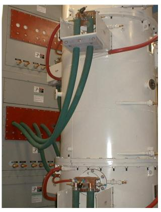
4.5m long, 3 zone 250mm ID, graphite tube 2200°C, water cooled
