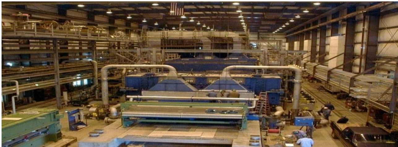
Harper LT : ~5.2 meter wide tow system in final assembly, Two (2) muffles 2.6 meter each
