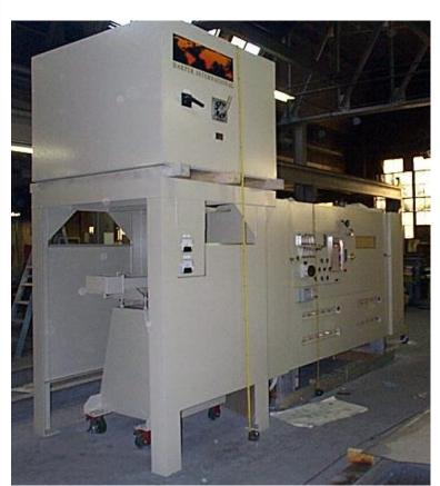
Width: 152mm / 6 inches Heated Length: 1524 mm / 60 inches Maximum Temperature: 2800°C
