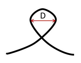
$$\begin{split} D_{Loop} \sim & \left(\frac{d}{\epsilon}\right)_{Fiber} = \left(\frac{d*E}{\sigma}\right)_{Fiber} \\ d = fiber \ diameter, \\ E = Modulus, \\ \sigma = tensile \ strength, \\ \epsilon = strain \ to \ failure \end{split}$$
