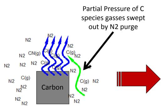
Near Stagnant N2 in heating chamber reduces carbon loss
