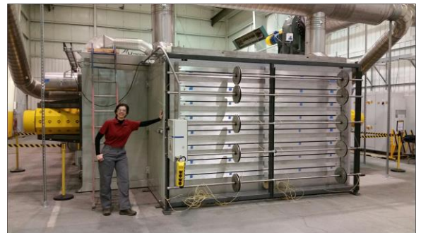
Shown Above: One section of Harper's Production Scale Oxidation Oven
