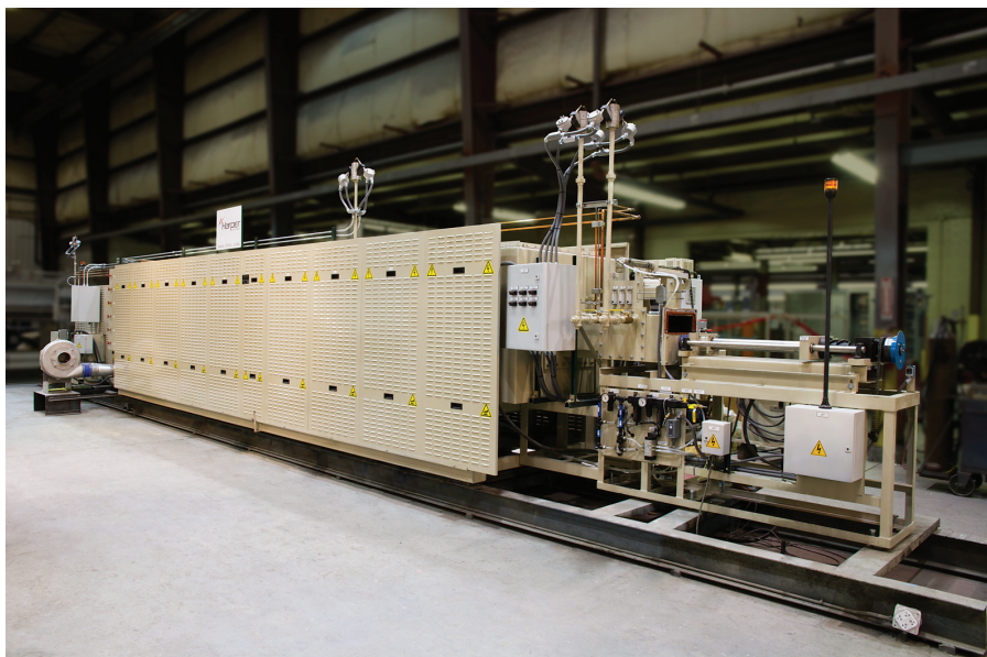
Fig. 2 Harper nuclear fuel sintering pusher furnace
