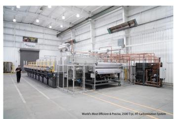
Harper's new on-line cleaning system, located in the entrance section, enables cleaning while the furnace is hot, resulting in increased HT Furnace run-time.
