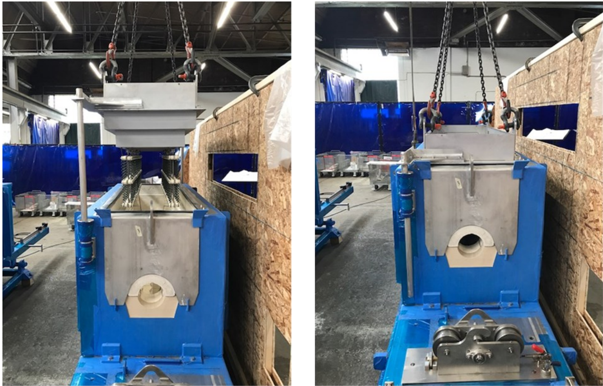
Figure 6. Assembly of the heating element into the rotary kiln
