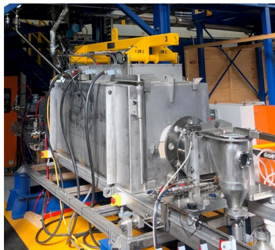
Figure 7. Harper Rotary Calciner within the ANSTO Synroc Demonstration Plant
