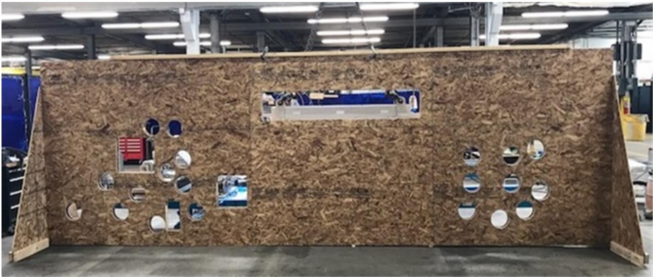
Figure 5. Mock Shield Wall for Rotary Calciner Testing
