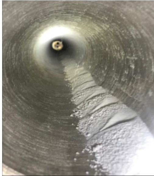
Figure 8. Calcined powder with waste stimulant from the unit integrated within Synroc's inactive engineering demonstrator
